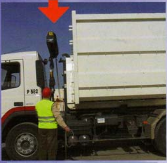
8 Using the control box, lower Hy-Tower to its fully retracted position.
